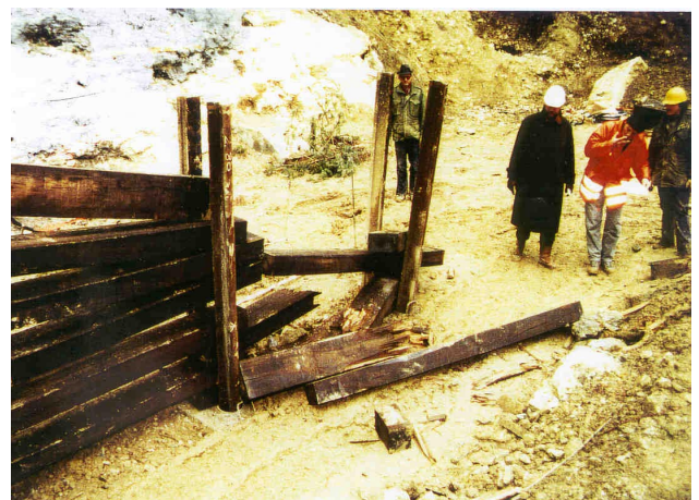
Fig. 5: Rockfall tests on a rail- and tie wall near Egerkingen, Switzerland, 1992.
