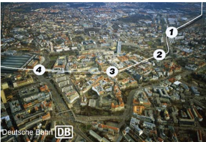
Fig.1: Alignment of the City-Tunnel Leipzig including the stations 1 – Bayerischer Bahnhof, 2 – Wilhelm-Leuschner-Platz, 3 – Markt, 4 – Main Station
